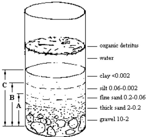
Figure 1 - Test for the composition of the soil.
